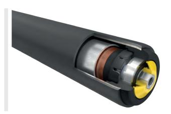
The PU sleeve ensures a high level of noise reduction, particularly for steel containers, and offers a high level of protection of sensitive materials. An improved conveyance of materials is achieved with the higher coefficient of friction compared with a steel tube. Materials can easily be separated since the larger diameter leads to a higher speed with the same rotational speed. With mechanical stress, e.g. with abrasion, it offers a higher robustness than a PVC sleeve.
