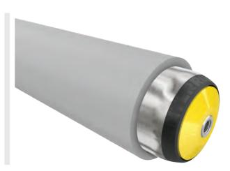
The PVC sleeve ensures a particularly high noise reduction and offers a high level of protection for sensitive materials. An improved conveyance of materials is achieved with the higher coefficient of friction compared with a steel tube. Materials can easily be separated since the larger diameter leads to a higher speed with the same rotational speed.
