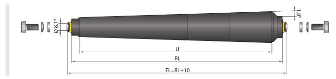
\* The recommended profile holes have a dimension of Ø 8.1 mm
