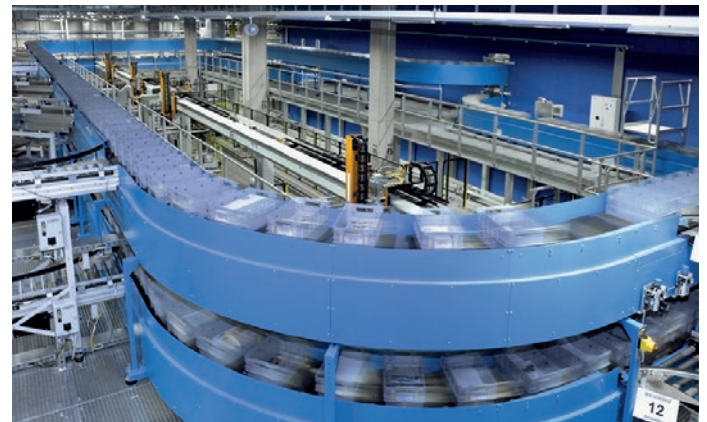
Space-saving double structure of Interroll's 12 Horizontal Crossbelt Sorters installed at SwissPost's three sorting centers in Switzerland.
