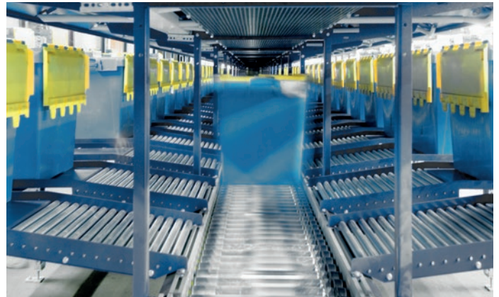
Space saving: a central take-away conveyor for full containers could be installed inside the vertical sorter.
