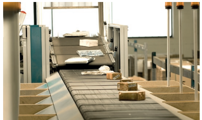
Interroll Vertical Crossbelt Sorter at DHL/Greven with 64 custom-made chutes, accessible from both sides
