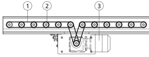
With wrapped force transmission, every conveyor roller is connected to the next one by a chain (1). For this reason the conveyor rollers require double sprocket heads (2). They need more space than with a tangential drive, so that the installation length of the roller is longer. Double sprocket heads always feature a DIN gearing (standard gearing).
