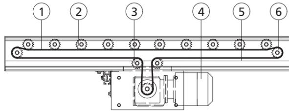
The tangential chain drive is characterized by its good level of efficiency and simple design. The drive head (2) consists only of one sprocket. For this reason, the installation length of the conveyor roller is shorter for a roller-to-roller drive. A single chain (1) drives all of the rollers in a conveyor. The chain is guided to the sprockets by a chain guide profile. The chain guide profile (5) is usually made of special plastic and must guide the chain extremely precisely.
