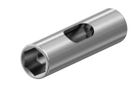
The fastening socket is used for tightening according to the torque of the RollerDrive fastening nut using a torque wrench. The socket features a lateral opening through which the RollerDrive connecting cable can be fed to the outside.
