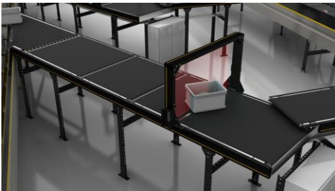
Image 2: The new generation of Interroll infeed conveyors (known as infeeds)
