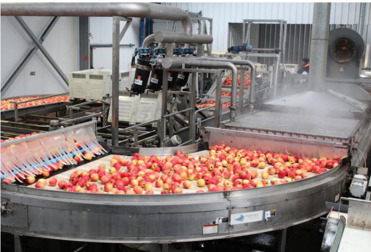
The Interroll Portec Belt Curve moving apples to the washing area.
